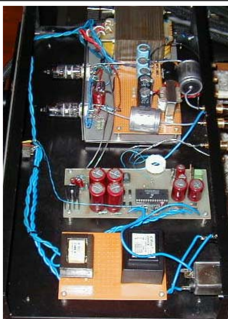
TDA1543 DAC with tube output stage
