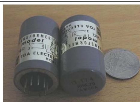
TOA 150:50k Mic Step-up Transformers
