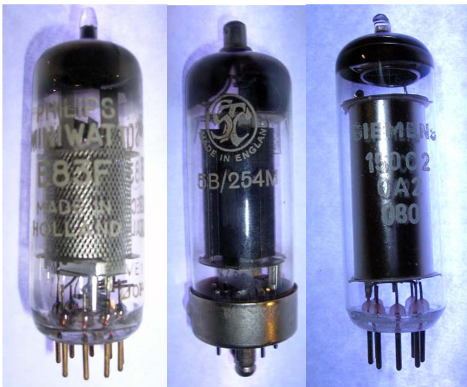
หลอด E83F Signal Pentode, 5B/254M Power Pentode and 0A2 Voltage Reference
