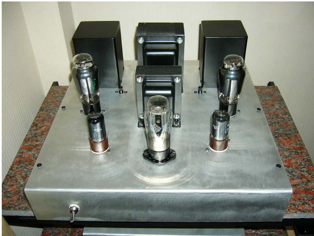
R120 Single-ended Amplifier, drive by CV1988
