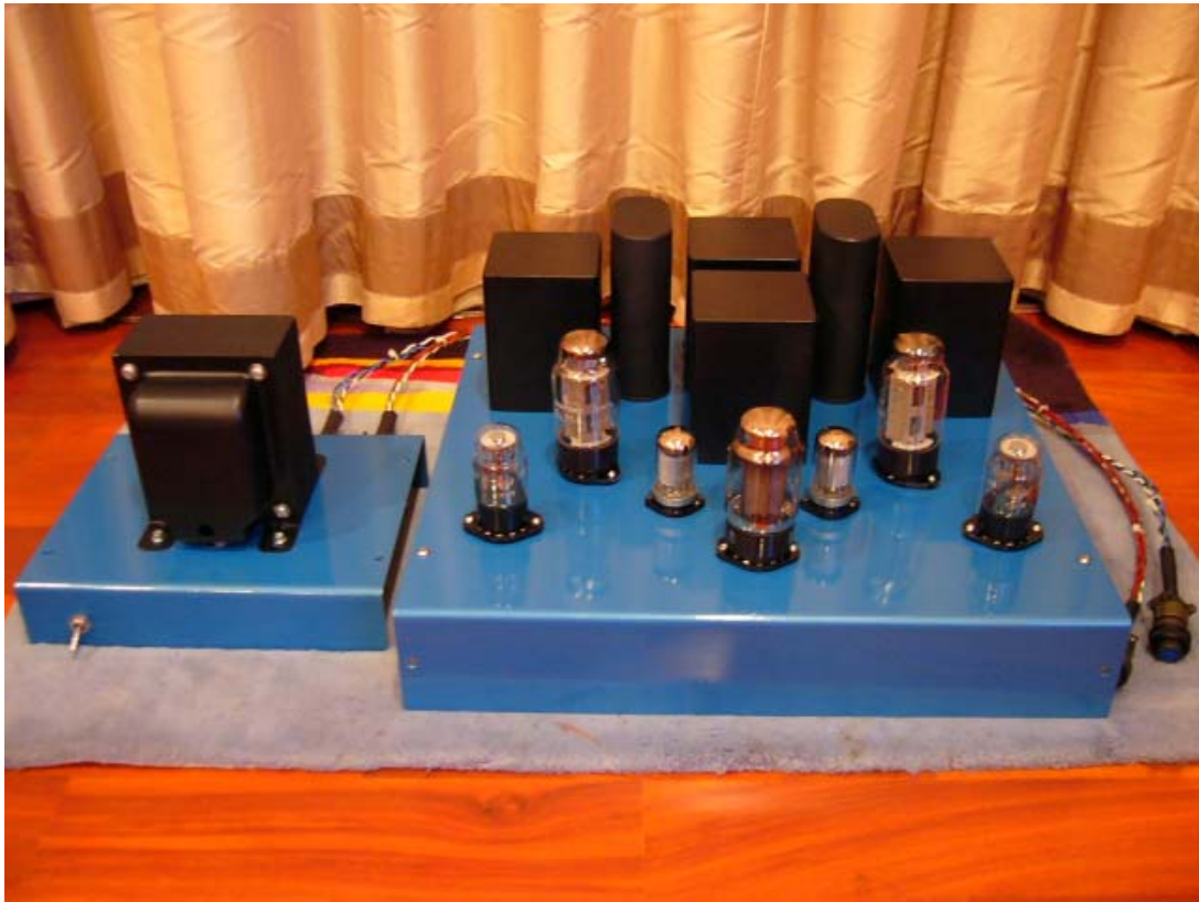
EL156 Power Pentode drive by C3m SE Amp
