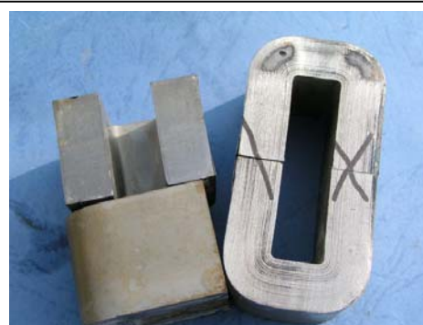
Supermalloy (Permalloy) 78% Ni 2% Co C-Core
