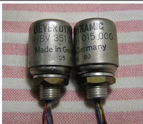
Beyer Dynamic 1 : 15 Step-up Transformer
