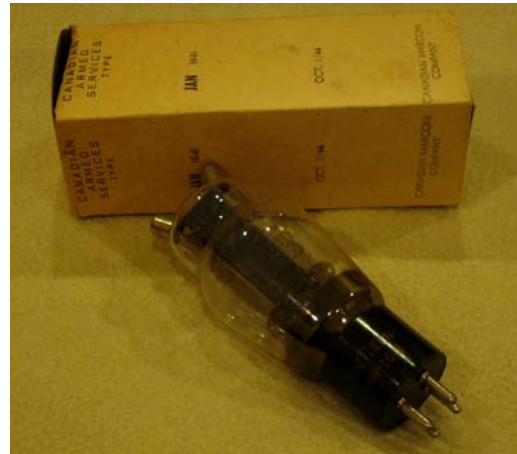
Raytheon RK-61 (1641) Full-wave Rectifier
